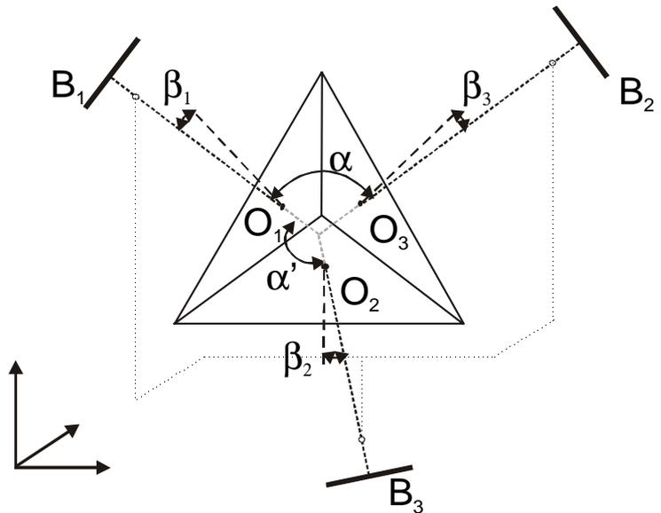
Fig. 5: Angular relationships for cubic signals
