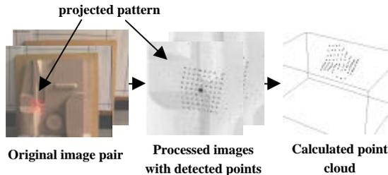
Figure 1. From a projected pattern to a point cloud
