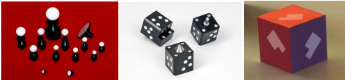
a) Retro-reflective sphere targets (GMS) b) Cubes with point coding (AICON) c) Color coded cube (i3mainz)
