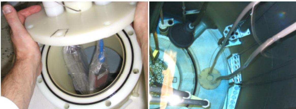
Figure 8: Left: Polyethylene container which carries camera and radiation sensor. Right: Top view of the reactor core with PE container. A 6 m water column protects people against radiation.
