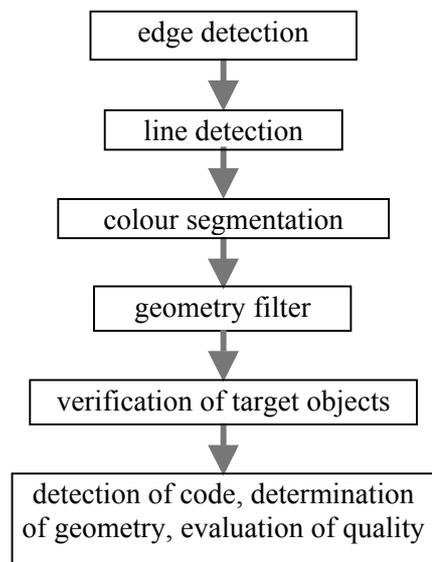
Fig. 6: structure of target detection
