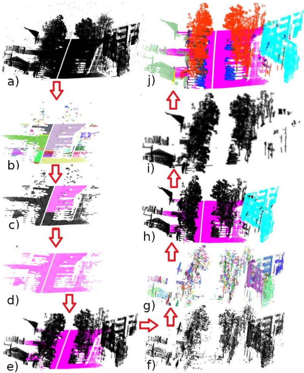
**Abb. 3:** The result of the object detection process step by step applied to a point cloud provided by Fraunhofer IPM
