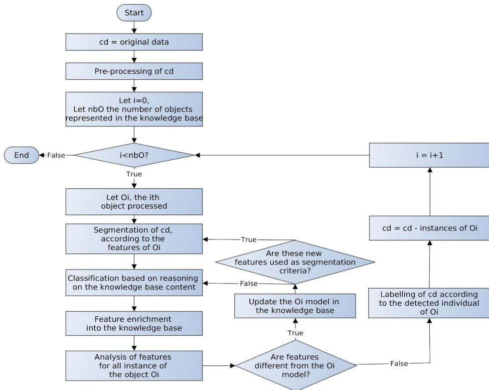
Abb. 2: Workflow of the overall process
