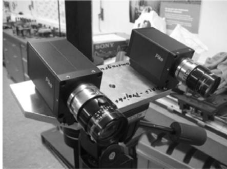
Figure 6. stereo configuration, with AVT cameras, type Pike
