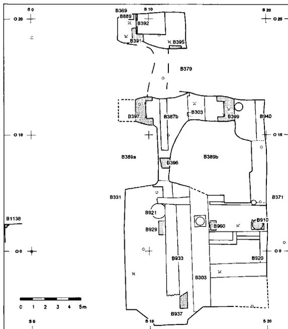
*Figure 7 Documentation of Roman wall remains underneath the present Cologne Cathedral. Visible remains shown as raster pattern filled areas*
