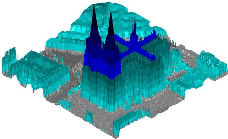
*Figure 8 Cologne cathedral, view generated from airborne laser scanner data (Source: TopScan)*
