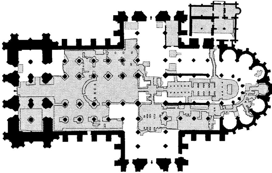
*Figure 2 Footprint of Cologne Cathedral with opened excavation areas shown as raster pattern filled areas*
